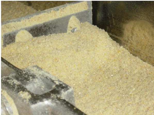
Residues in chain conveyer
